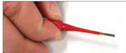
Plastic tool with contact in proper position.
