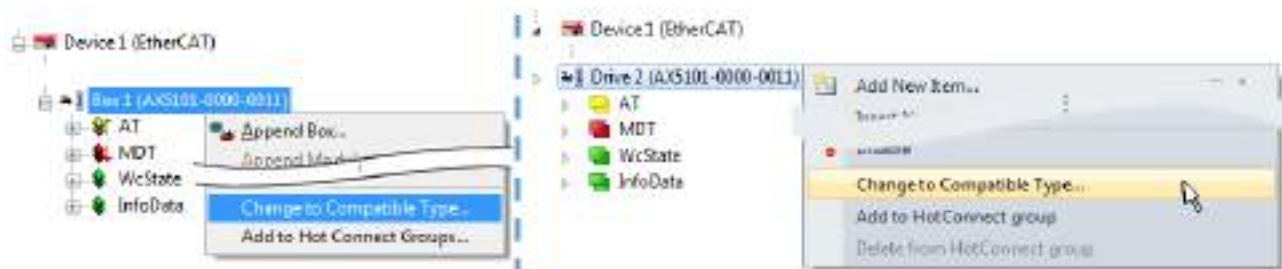
Fig. 74: Dialog “Change to Compatible Type...” (left: TwinCAT 2; right: TwinCAT 3)
