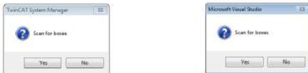
Fig. 62: Scan query after automatic creation of an EtherCAT device (left: TwinCAT 2; right: TwinCAT 3)
