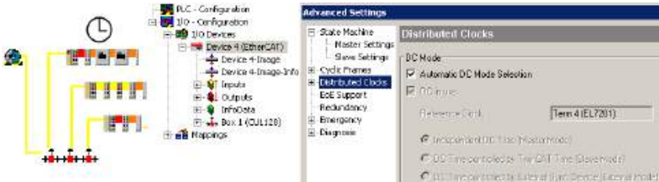
Fig. 95: example topology with EL7201 as reference clock
