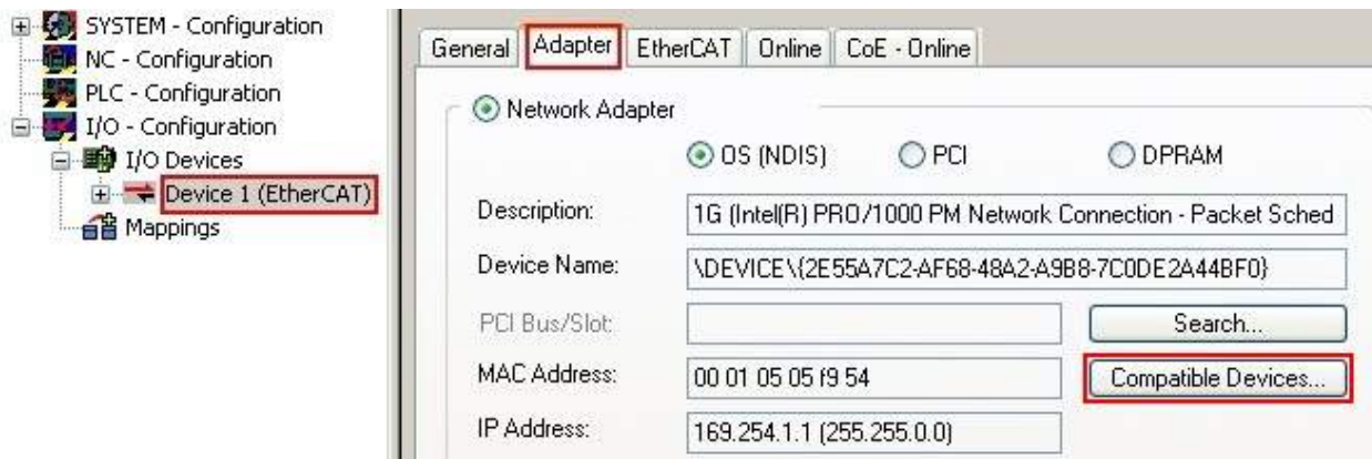
Fig. 34: EtherCAT device properties(TwinCAT 2): click on “Compatible Devices...” of tab “Adapte”
