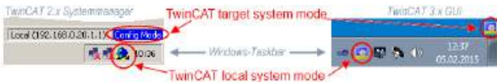
Fig. 55: Differentiation local/target system (left: TwinCAT 2; right: TwinCAT 3)
