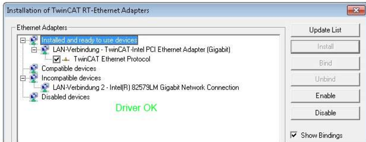
Fig. 36: Exemplary correct driver setting for the Ethernet port
