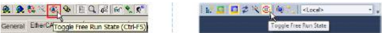
Fig. 67: TwinCAT can also be switched to this state by using a button (left: TwinCAT 2; right: TwinCAT 3)
