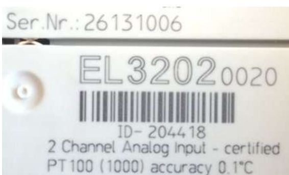
Fig. 29: EL3202-0020 with serial/ batch number 26131006 and unique ID-number 204418
