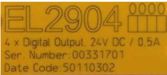
Fig. 32: EL2904 IP20 safety terminal with batch number/ date code 50110302 and unique serial number 00331701
