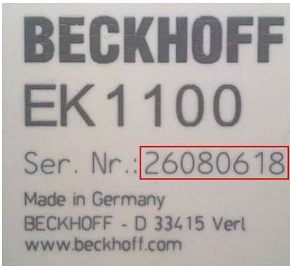
Fig. 27: EK1100 EtherCAT coupler, standard IP20 IO device with serial/ batch number
