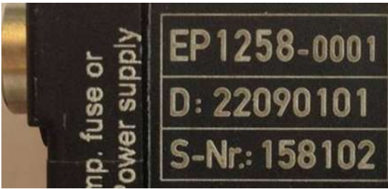
Fig. 30: EP1258-00001 IP67 EtherCAT Box with batch number/ date code 22090101 and unique serial number 158102
