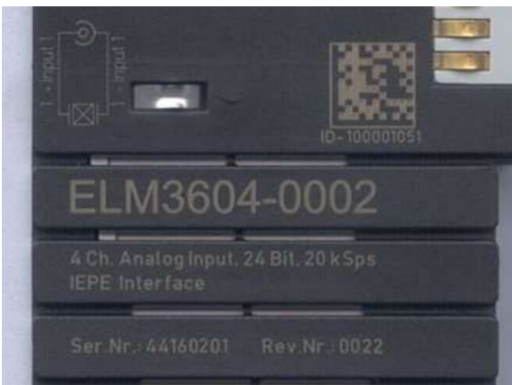
Fig. 33: ELM3604-0002 terminal with unique ID number (QR code) 100001051 and serial/ batch number 44160201
