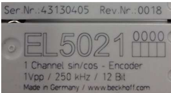
Fig. 26: EL5021 EL terminal, standard IP20 IO device with serial/ batch number and revision ID (since 2014/01)
