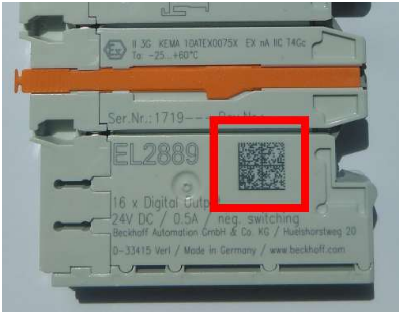
Fig. 34: BIC as data matrix code (DMC, code scheme ECC200)
