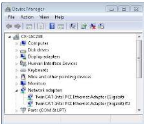
Fig. 30: Windows 7, identification of the Ethernet interfaces (X000, X001) in the device manager.
