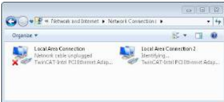
Fig. 29: Windows 7, Identification of the Ethernet interfaces (X000, X001) in the Network and Sharing Center.
