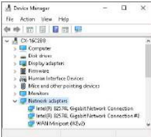
Fig. 32: Windows 10, identification of the Ethernet interfaces (X000, X001) in the device manager.
