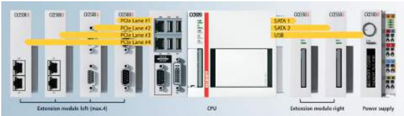
Fig. 1: Overview of the CX2000 product family with basic CPU module, power supply unit and modules.
