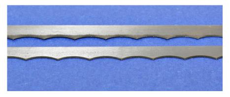
The 1/2 inch pitch blades are the most common and are used for soft white and wheat breads.
