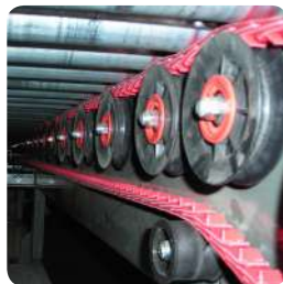
PowerMax V-Belt Idlers used with POWERVIST Roller Drive on a Live Roller Conveyor.
