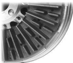
Cross-drilled rotor with heat dissipating fins.
