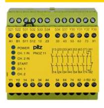
Safety relay (standalone), inputs: 1/2-channel wiring with/without detection of shorts across contacts, outputs: 7 N/O, 1 N/C,1 SC, automatic/manual/monitored start, start-up test, UB = 110 - 120 V AC/24 V DC, width: 90 mm, screw terminals integrated, monitoring of E-STOP, safety gates, feedback loop.
