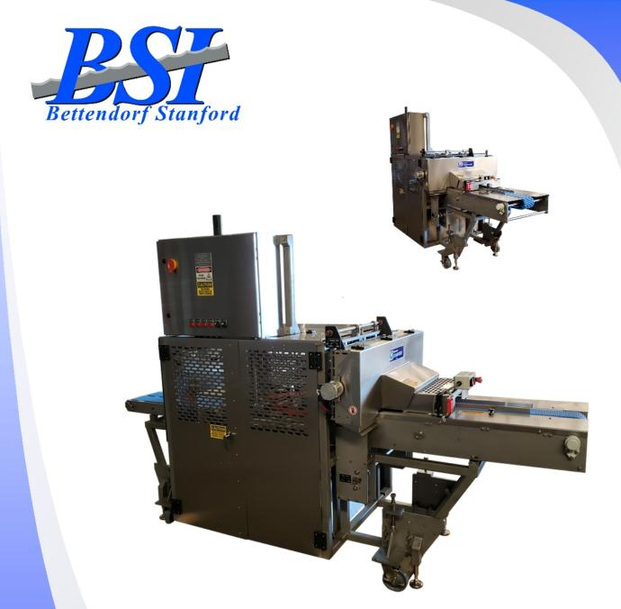
Frozen roll slicer for sandwich assembly. This slicer will slice a single row of frozen rolls such as English muffins, ciabatta, biscuits, or croissants at temperatures as low as 0 degree internal temp. After slicing, the rolls are separated so that the tops are sitting next to the bottoms for easy sandwich assembly.
