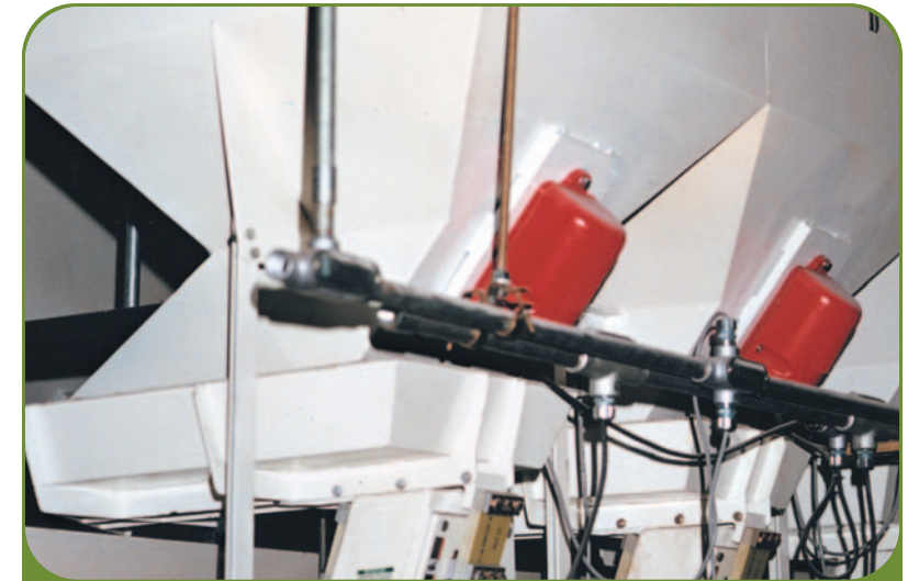
Syntron® model V-20 Electromagnetic Vibrators maintain the flow of pasta from bins to packaging lines.
