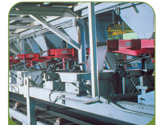
Ideal for controlling bulk material in mixing, blending, batching, grinding and packaging operations, the ten standard Light Industry Electromagnetic Vibrating Feeder models operate with maximum capacities ranging from 1,250 pounds to 25 tons per hour, based on material weighing 100 pounds per cubic foot.
